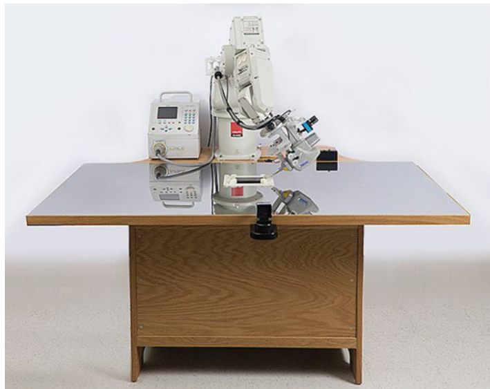
Figure 77 — Robotic IEC 61000-4-2 Test System
