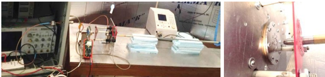
Figure 107 — Test Setup of the Air Discharge Experiment [Li2017]
